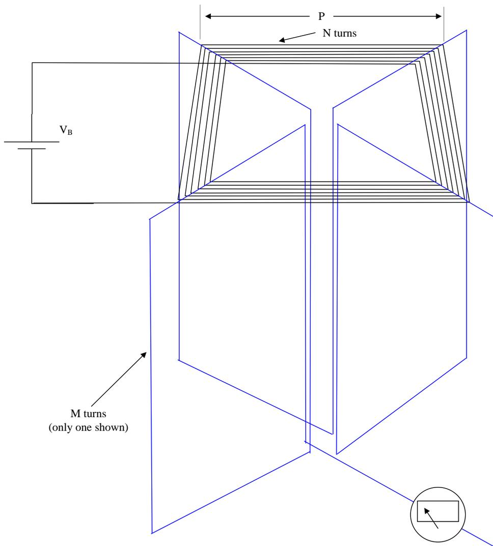
Figure 11-1: Corner Effect Transformer
