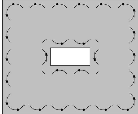
**Figure 8-3 Effective current of magnet with hole.**
