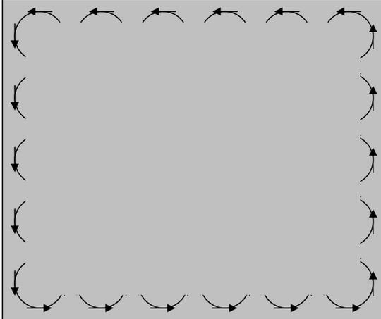
**Figure 8-2: Effective current (Edge Current)**
