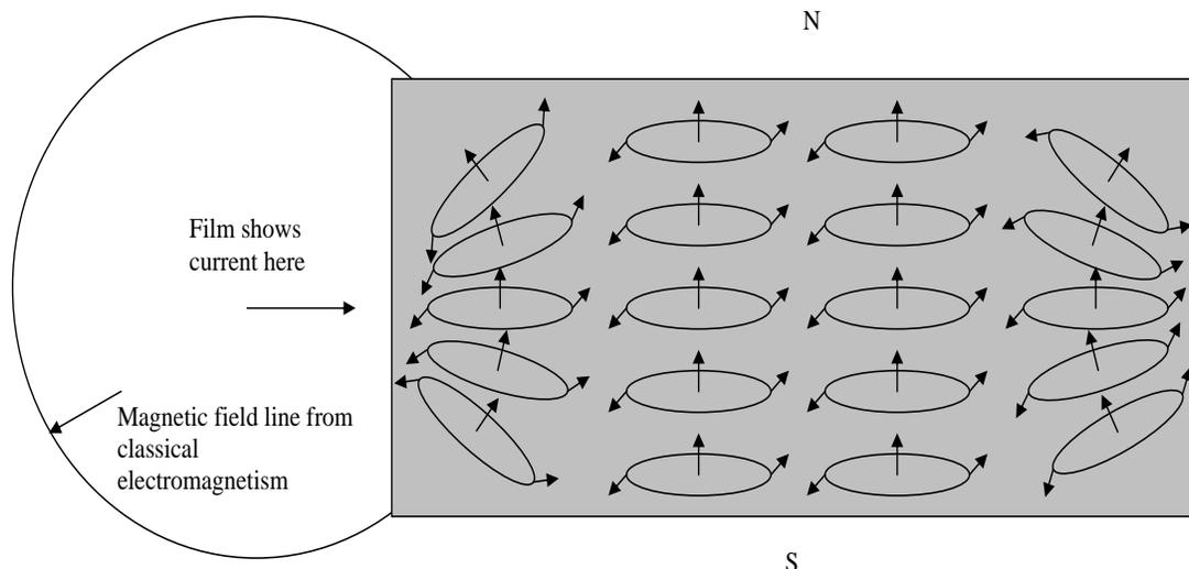
**Figure 8-10: Edge current of single magnet.**
